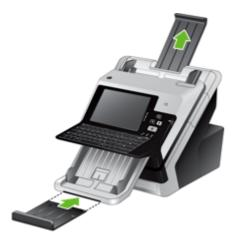
Adjust the paper guides to the width of the documents. Take care not to overtighten the guides, which can restrict paper feeding.
